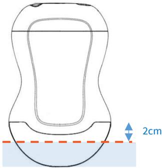
Figure 11 : Immersion limit of echOpen O1 probe
